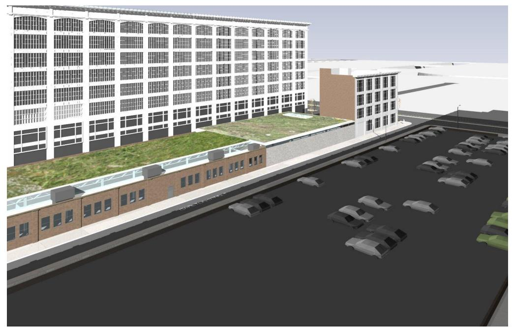
The renovated shed building and Studio Building will feature a green roof system that will aid in controlling the temperature of the spaces as well as provide an attractive roofscape to surrounding buildings.
