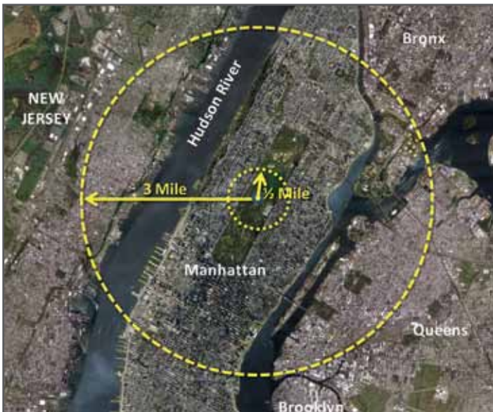
Comparison of Minimum Curve Radii: Next-Gen High-Speed Rail and 65-mph Commuter Alignments
