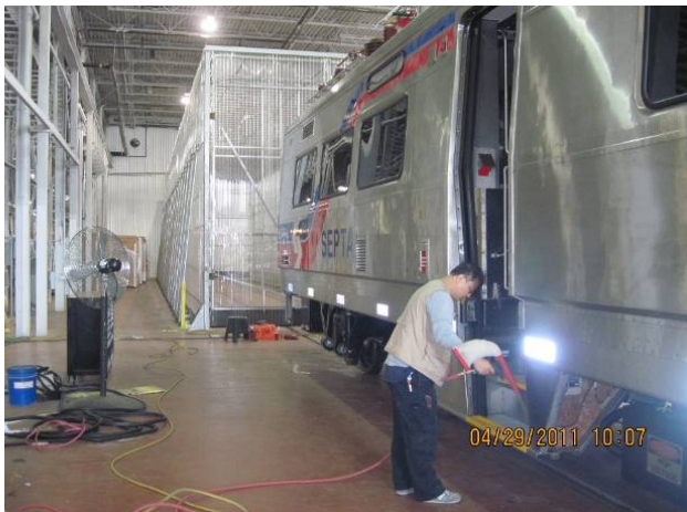
Car 811 during preparations for water testing
