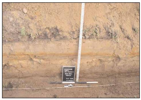
**Photograph 37:** Shot of west wall profile GeoTrench 8 125-130 feet showing modern fill over modern alluvium (banded sands) over Pleistocene-aged soil with cobbles. View facing west (May 2008).
