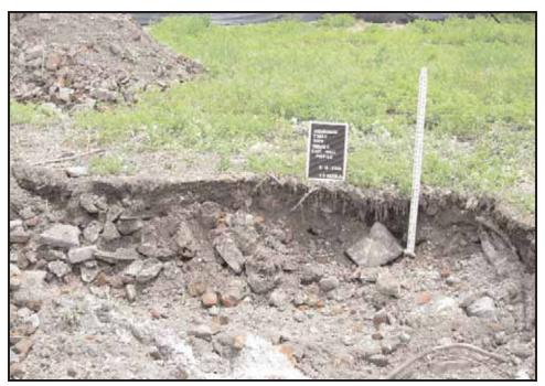
**Photograph 12:** Shot of east wall profile of Beach Street Power Station Trench 2 showing demolition fill and impenetrable steel reinforced concrete in Historic Area H-1. View facing east (May 2008).
