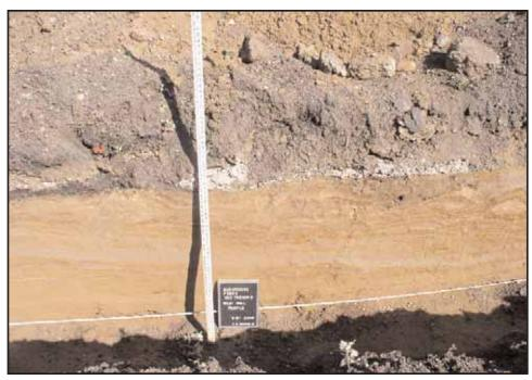
**Photograph 41:** Shot of west wall profile GeoTrench 9 24-34 feet showing modern fill over modern alluvium (banded sands) over Pleistocene-aged soil with cobbles. View facing west (May 2008).
