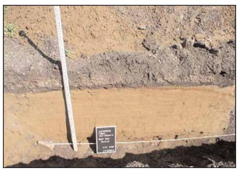
**Photograph 40:** Shot of west wall profile GeoTrench 9 2-9 feet showing modern fill over modern alluvium (banded sands) over Pleistocene-aged soil with cobbles. View facing west (May 2008).
