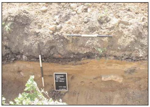
**Photograph 29:** Shot of east wall profile GeoTrench 7 86-94 feet showing modern fill horizons over modern alluvium (banded sands) over Pleistocene-aged soils with cobbles. View facing east (May 2008).
