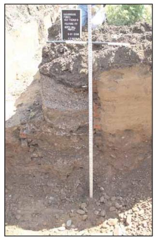
**Photograph 53:** Profile shot of Feature 177 in Historic Area H-2 showing layers of coal ash and ash fill throughout. View facing north (May 2008).
