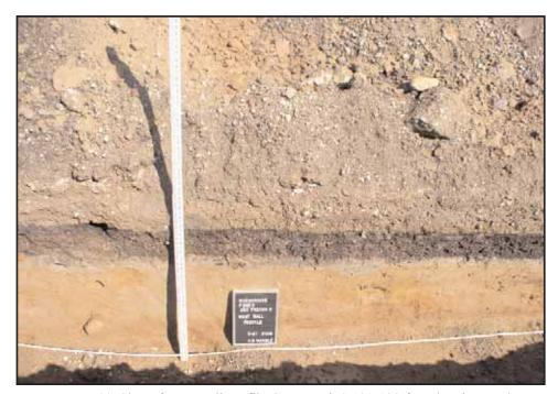
**Photograph 44:** Shot of west wall profile GeoTrench 9 121-130 feet showing modern fill over modern alluvium (banded sands) over Pleistocene-aged soil with cobbles. View facing west (May 2008).
