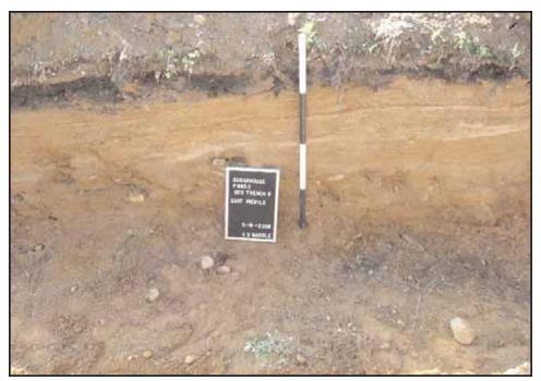
**Photograph 24:** Shot of east wall profile GeoTrench 6, 99-108 feet showing fill horizons over modern alluvium (banded sands) over Pleistocene-aged soils with cobbles. View facing east (May 2008).
