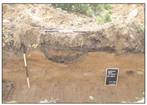
**Photograph 30:** Shot of east wall profile GeoTrench 7 102-110 feet showing modern fill horizons over modern alluvium (banded sands) over Pleistocene-aged soils with cobbles. View facing east (May 2008).
