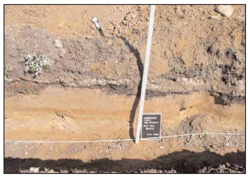
**Photograph 43:** Shot of west wall profile GeoTrench 9 67-74 feet showing modern fill over modern alluvium (banded sands) over Pleistocene-aged soil with cobbles. View facing west (May 2008).
