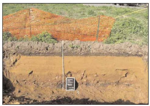
**Photograph 16:** South wall profile shot of GeoTrench 3 showing layers of modern fill over banded alluvium and Pleistocene-aged subsoil. View facing south (May 2008).
