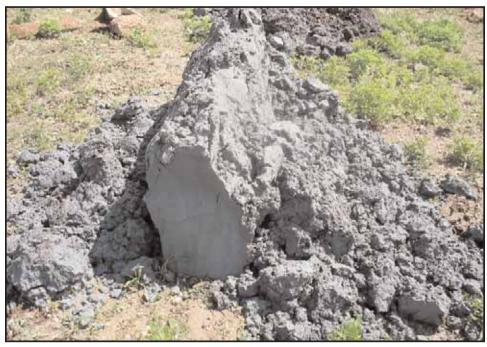
**Photograph 65:** An example of the gley-colored, riverine soils reached at 12 feet below surface in SRT-2 (May 2008).
