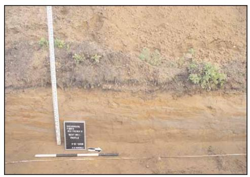
**Photograph 36:** Shot of west wall profile GeoTrench 8 78-86 feet showing modern fill over modern alluvium (banded sands) over Pleistocene-aged soil with cobbles. View facing west (May 2008).
