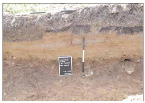
**Photograph 23:** Shot of east wall profile GeoTrench 6 54-62 feet showing modern alluvium (banded sand) overlying Pleistocene soil with cobbles. View facing east (May 2008).
