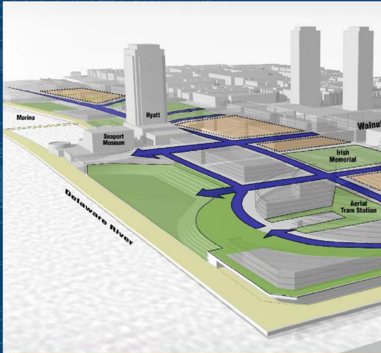
Diagram of potential infrastructure improvements - extended street grid, park space (green), and I-95 covering (orange)
